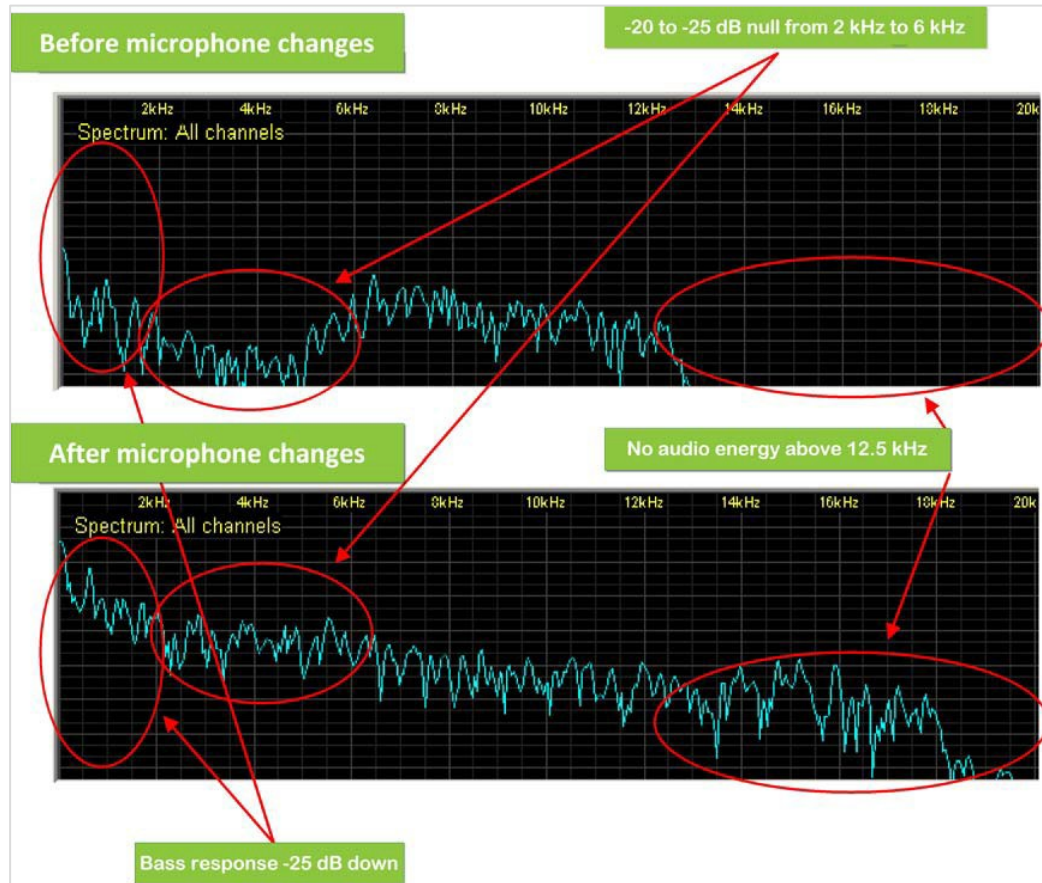
Figure 14 – Audio Spectrum Before and After Microphone Replacement and Equalizer Adjustments
