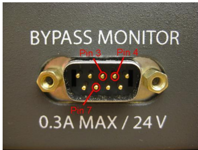
Figure 5: DB9 Pinouts for Remote Bypass Monitoring
