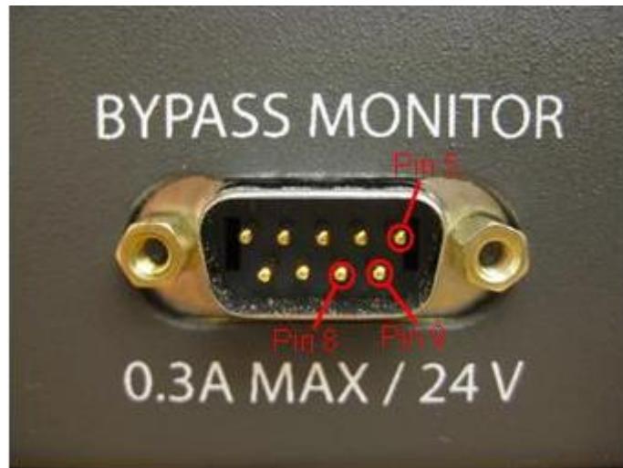
Figure 7: DB9 Pinouts for Remote Alarm Status Monitoring
