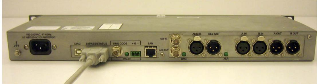
**Figure 11: Rear Panel DE-9 M Connection**
