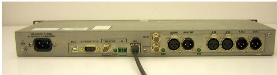
**Figure 10: Rear Panel Ethernet Connection**
