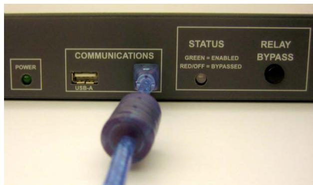
Figure 16: Front Panel USB Type B Connection
