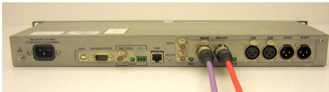
Figure 9: Rear Panel Digital XLR Connections
