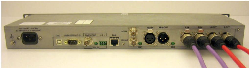
Figure 6: Rear Panel Stereo Analog XLR Inputs and Outputs
