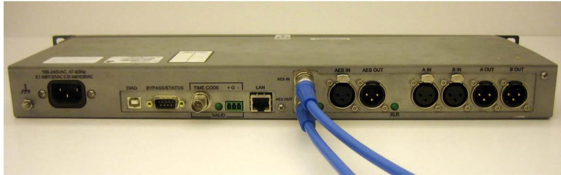
Figure 8: Rear Panel Digital BNC Connections
