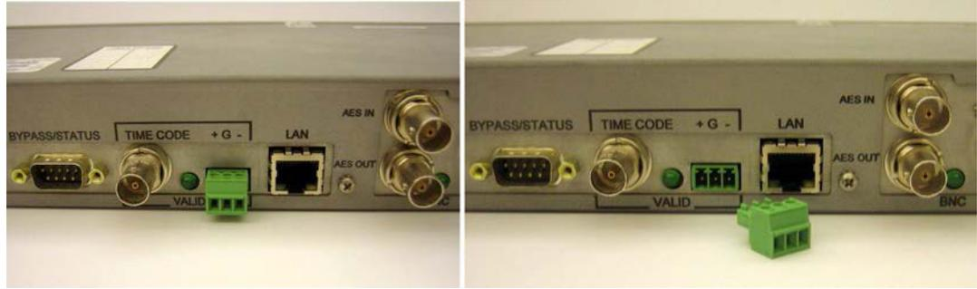
**Figure 13: Quick Disconnect Plug in Socket (Left) and out of Socket (Right)**
